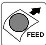
Use this button to feed paper or to start self test and for hexadecimal dump mode. (See the instructions "Self test" (8) in this chapter for self test.) (See the instructions "Hexadecimal dump" in Chapter 9 for hexadecimal dump mode.)
