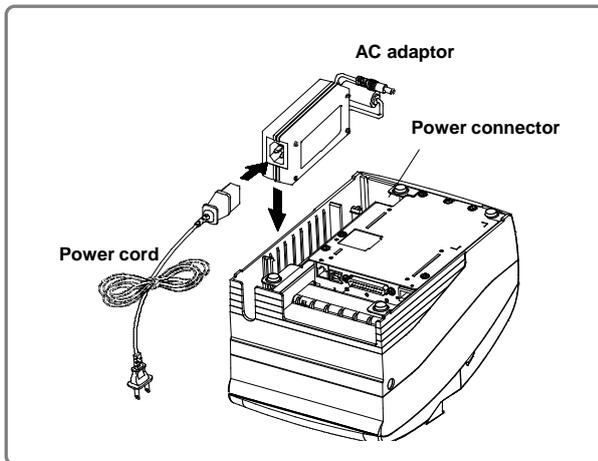
• **Connect the AC adapter according to the following procedure.**
