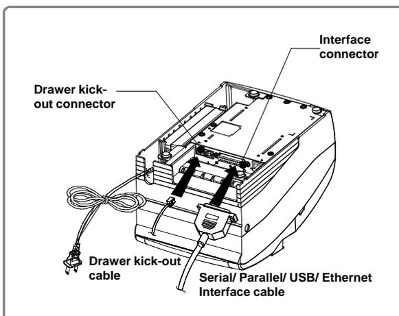
• **Connect the cables according to the following procedure.**
