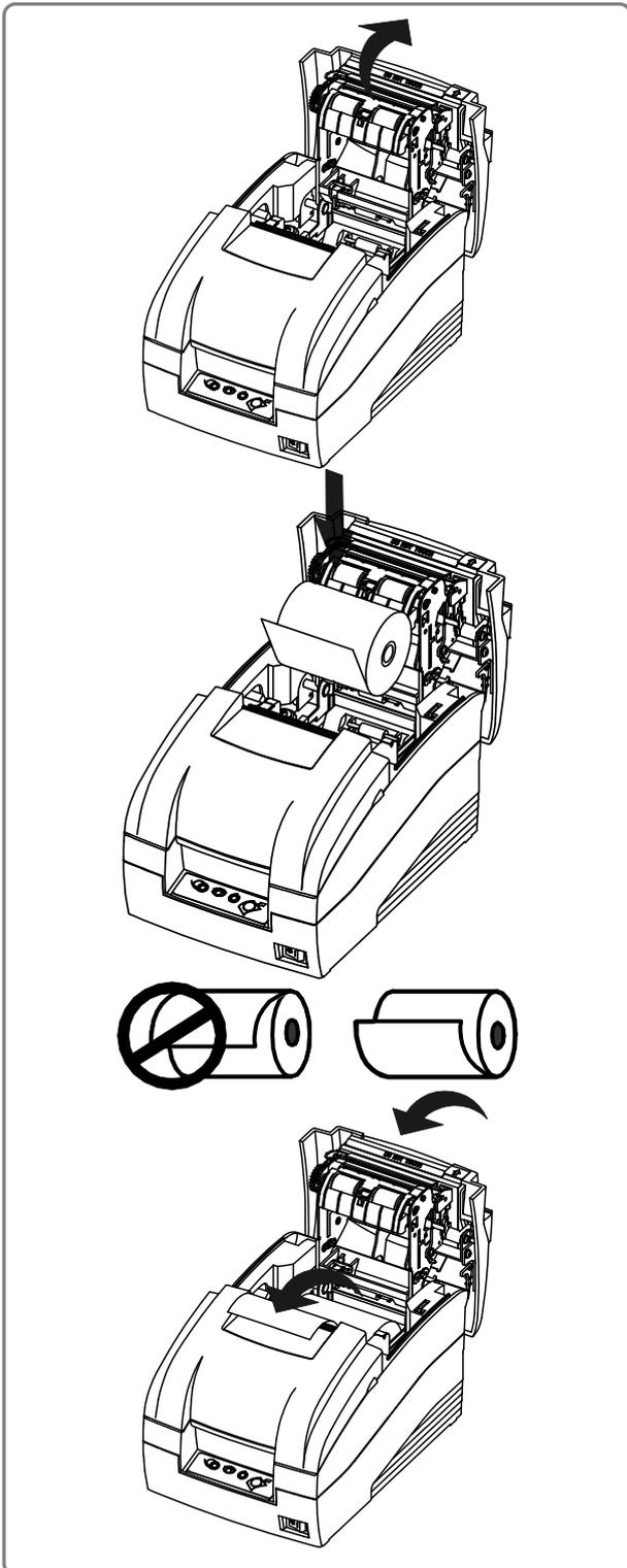
1) Open the rear cover by pushing the open button.
