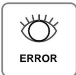
When this indicator light is on (but not blinking), it means that the printer is out of paper or almost out of paper or the printer covers are open. When this light is blinking, there is an error. (See "ERROR LED blinking pattern" in Chapter 11.) If you see this light blinking, turn off the printer for a few seconds and then turn it back on. If the light is still blinking, call your supervisor or a service person.
