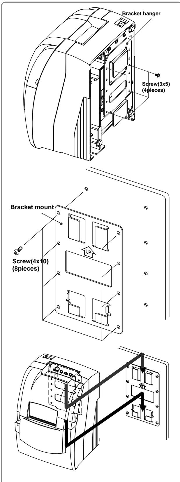
1) Turn the Set over and attach the Bracket hanger to the Frame base then tighten four screws.
