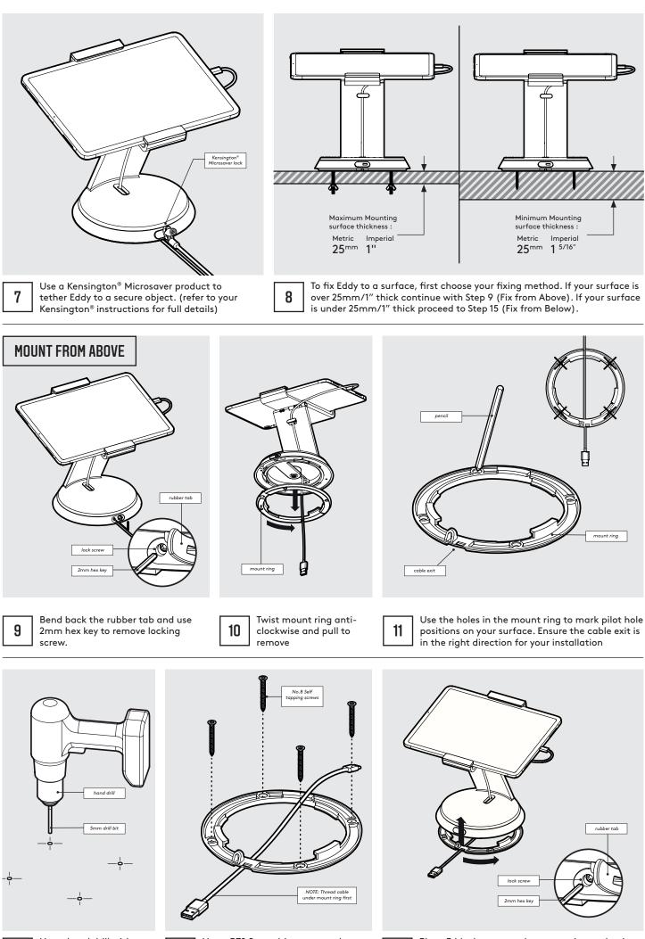
Use a hand drill with 4mm bit to make pilot holes in your surface.
