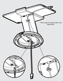
Feed your charge cable through the base and plug it into your tablet. Use the rubber hooks to keep it tidy.
