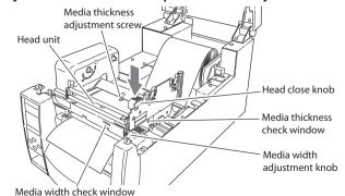
8. With the power switched on, push the FEED key to feed the media. It will halt at the next print start position.
