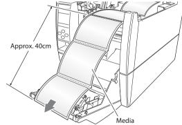
4. Peel off a number of labels at the tip part of the media from the liner so that the liner unit is in contact with the peeler roller when closing the rewinder cover.
