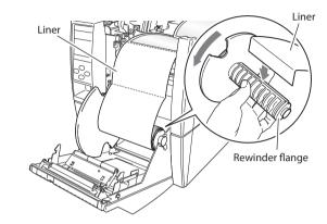
6. Confirm that the liner unit is in place in the peeler roller and close the rewinder cover.
