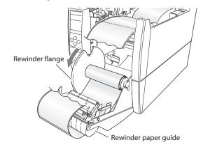
7. If the optional adjustable rewinder flange is being used with a paper core, the media can be attached to the paper core directly with tape or glue. Then the flange is set in the printer. For details on installing and removing the cardboard refer to the instructions contained with the adjustable flange.
