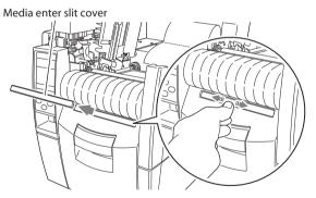
3. Open the rewinder cover and remove the rewinder flange.
