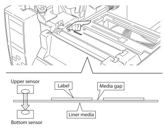
3. If the Pause Key is pressed then released while the MENU key is continually pressed, the sensor is automatically adjusted.
