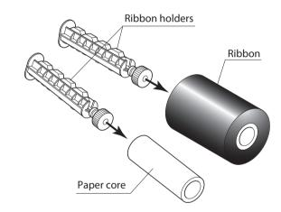
2. Install the unused ribbon and holder in to the rear ribbon drive unit. The splines on the ribbon drive gear mechanism engage with the end of the ribbon holder.
