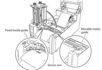
Lower the head unit back down to the closed position. Push the head close knob firmly to close and lock the mechanism. The mechanism is only locked correctly when you head a "click". Align it with the width of the media that has been set, then set the media width adjustment screw and the media thickness adjustment knob. See "Chapter 3 Printer Adjustments".
