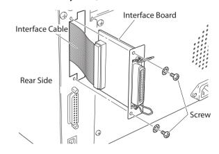
2. Remove the connecting cable from the interface board and reconnect the cable to the connector of the replacement interface board
