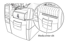
6. Insert the end of the media in to the slot in the rewinder flange and wind the media on to itself with two or three turns to ensure it is held properly. Set the rewinder flange back in to the printer.
