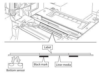
3. If the Pause Key is pressed then released while the MENU key is continually pressed, the sensor is automatically adjusted.
