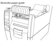
2. Slide the media enter slit cover above the rewinder cover to the left or right while pressing down on its center and remove.
