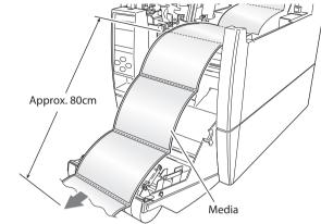
5. Insert the tip of the media through the media enter slit from the external side of rewinder cover.
