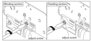
When turning adjust-screw, use a flat-tip screwdriver.
