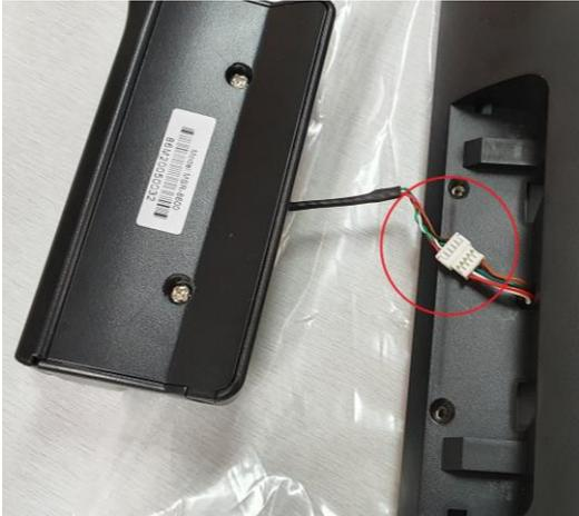
Step 3. Tighten two screws on the MSR.
