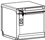
2. In the correct direction of the roll paper, install the roll paper.
