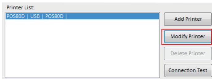
4. Choose "POS80D" for printer driver, choose "COM3" for system port, click "OK", so the printer is connected through BT.
