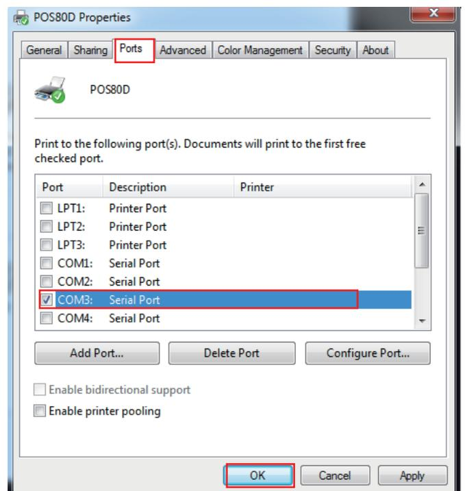
7. Choose "General" under "Printer properties" and click "Print Test Page" to print the test page. If the printing is failed, check whether Bluetooth is disconnected or the corresponding COM port is occupied.
