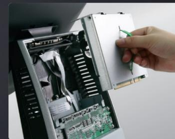
CPU module can be extracted for efficient upgrades and maintenance
