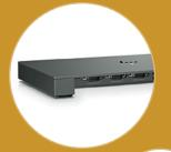
Gain optimum connectivity with two I/O connectivity base options that provide inputs such as serial, USB, PUSB, cash drawer, LAN, and video output (USB-C™)
