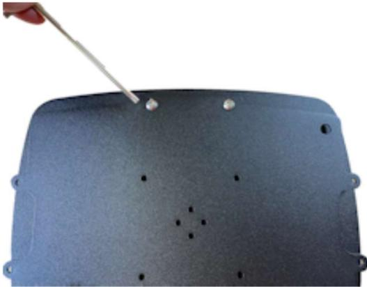
1. Remove the Screws from the back of the Frame and take off the back cover from the frame.
